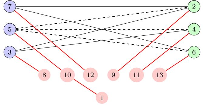
**Fig. 2** Reducing reconstruction of even-odd-bipartite graph to construction of BFS tree in even-odd-bipartite graphs: given the even-odd-bipartite graph  $G$  (with node set  $\{2, \dots, 7\}$ ), in order to check the edges of  $G$  incident to 5, we build the auxiliary graph  $G_5$  by adding nodes  $\{1, 8, \dots, 13\}$  as depicted on the figure. Node  $j \in \{2, 4, 6\}$  is in the third layer of a BFS-tree rooted in 1 if and only if  $(5, j)$  is an edge of  $G$ .
