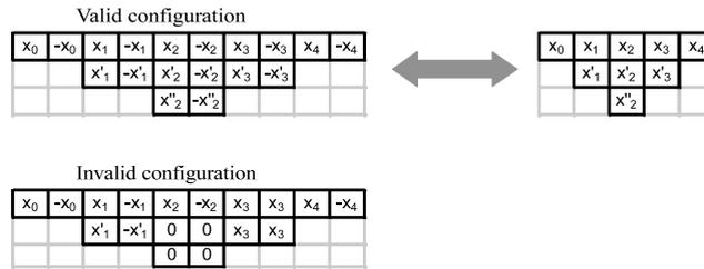
Fig. 2. Behavior of the NCCA: invalid pairs of cells remain constant, valid pairs in the presence of valid (local) configurations iterate according to the original rule, valid pairs in the presence of invalid configurations become 0.
