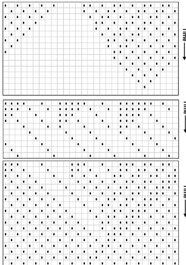
Fig. 4. Sample dynamics for rules 40 (top), 152 (center) and 184 (bottom), with periodic boundary condition.
