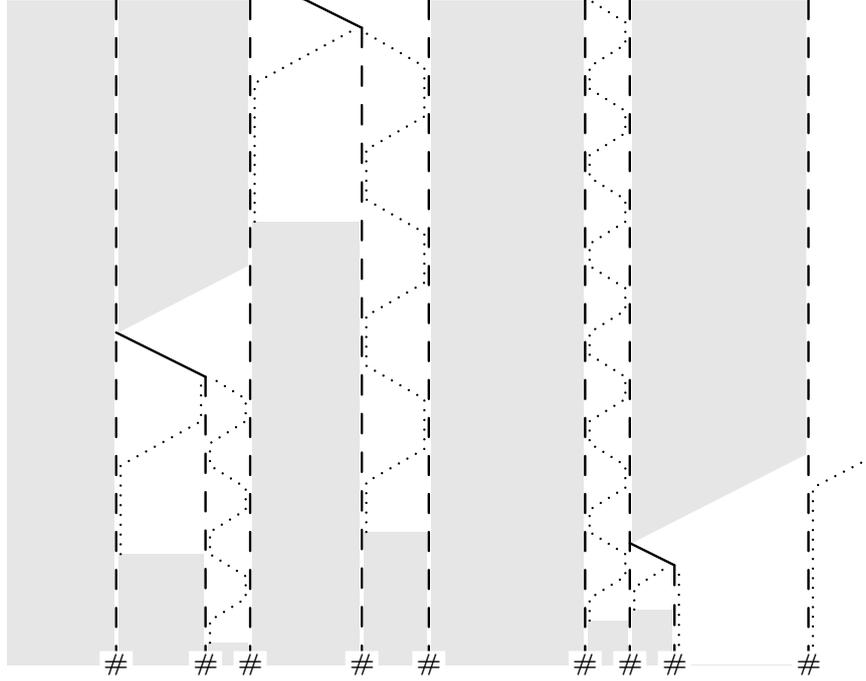
Figure 2: A  $\#$  stays until two segments merge. Computation happens in gray areas, and at its end a signal (...) is sent and stays on the left of the segment, then goes to the right, stays and comes back. This cycle continues until a neighbor's signal is on the same  $\#$  at the same time. Then the  $\#$  is deleted and another computation is started on the left.
