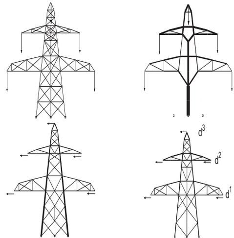
**Fig. 5** Electricity mast: ground structure, single-load solution and two minimum expected compliance counterparts.
