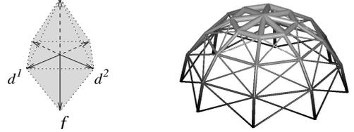
**Fig. 4** Dome: 2 orthogonal perturbations at the top and optimal solution.
