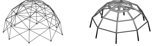
**Fig. 3** Dome: ground structure and single-load optimal solution.
