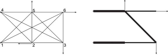
**Fig. 1** Toy example: ground structure and unstable optimal solution.
