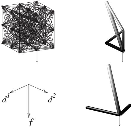
**Fig. 6** Ground structure, single-load solution and stable counterpart by considering 2 orthogonal perturbations.
